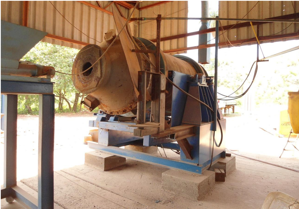
Mineração Tuiuiu - Brazil – Frontier/Four Star Producing gold by pyrometallurgy Poconé – MT – Rotary Smelter Furnace
