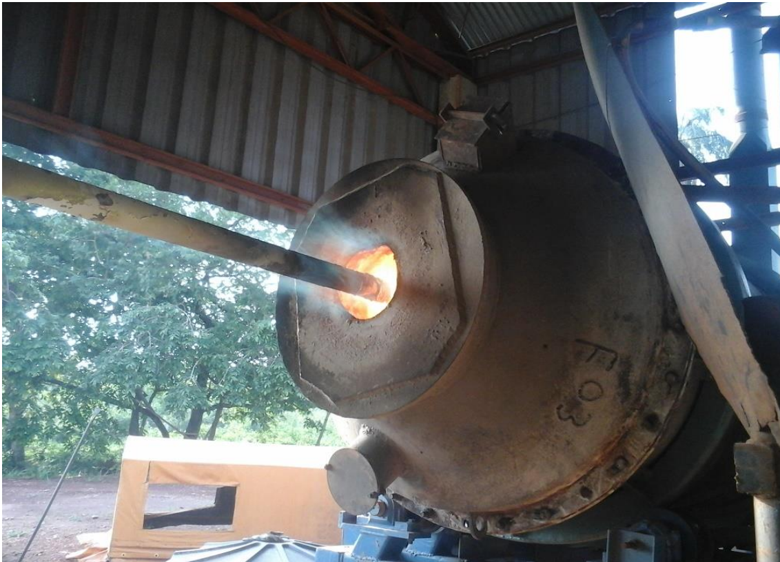
Mineração Tuiuiu - Brazil – Frontier/Four Star Producing gold by pyrometallurgy Poconé – MT – Smelter on fire
