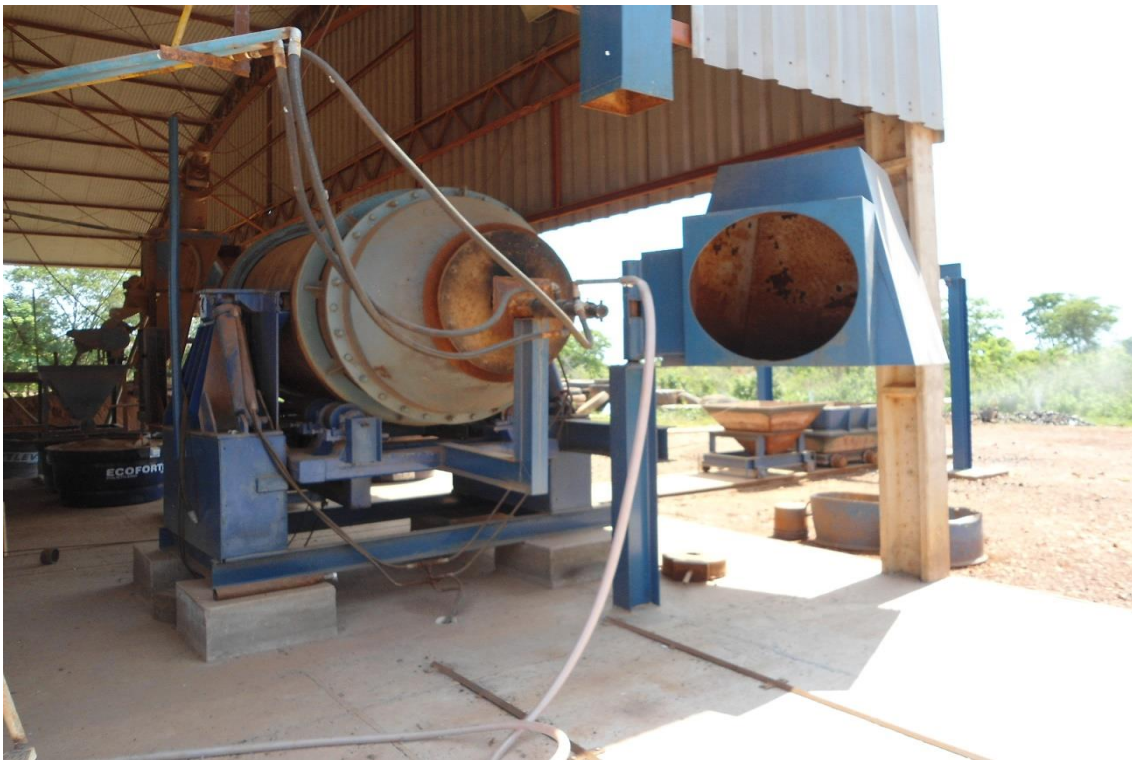
Mineração Tuiuiu - Brazil – Frontier/Four Star Producing gold by pyrometallurgy Poconé – MT – Front of Smelter
