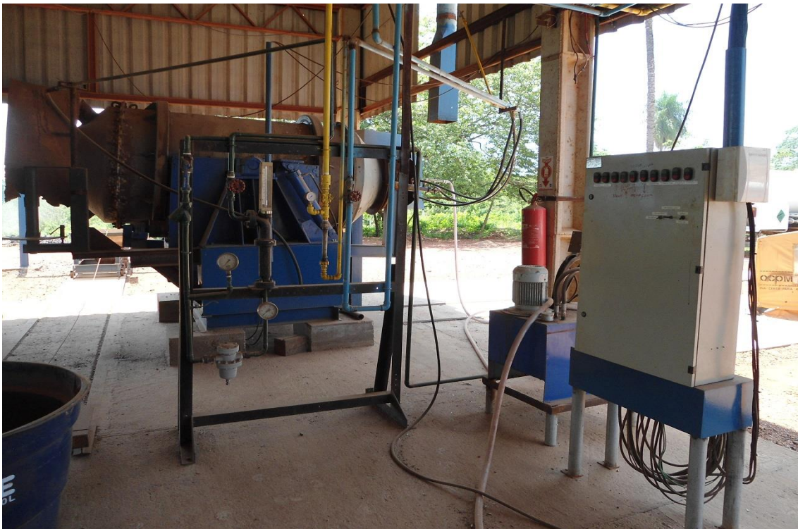
Mineração Tuiuiu - Brazil – Frontier/Four Star Producing gold by pyrometalurgy Field Control Panel
