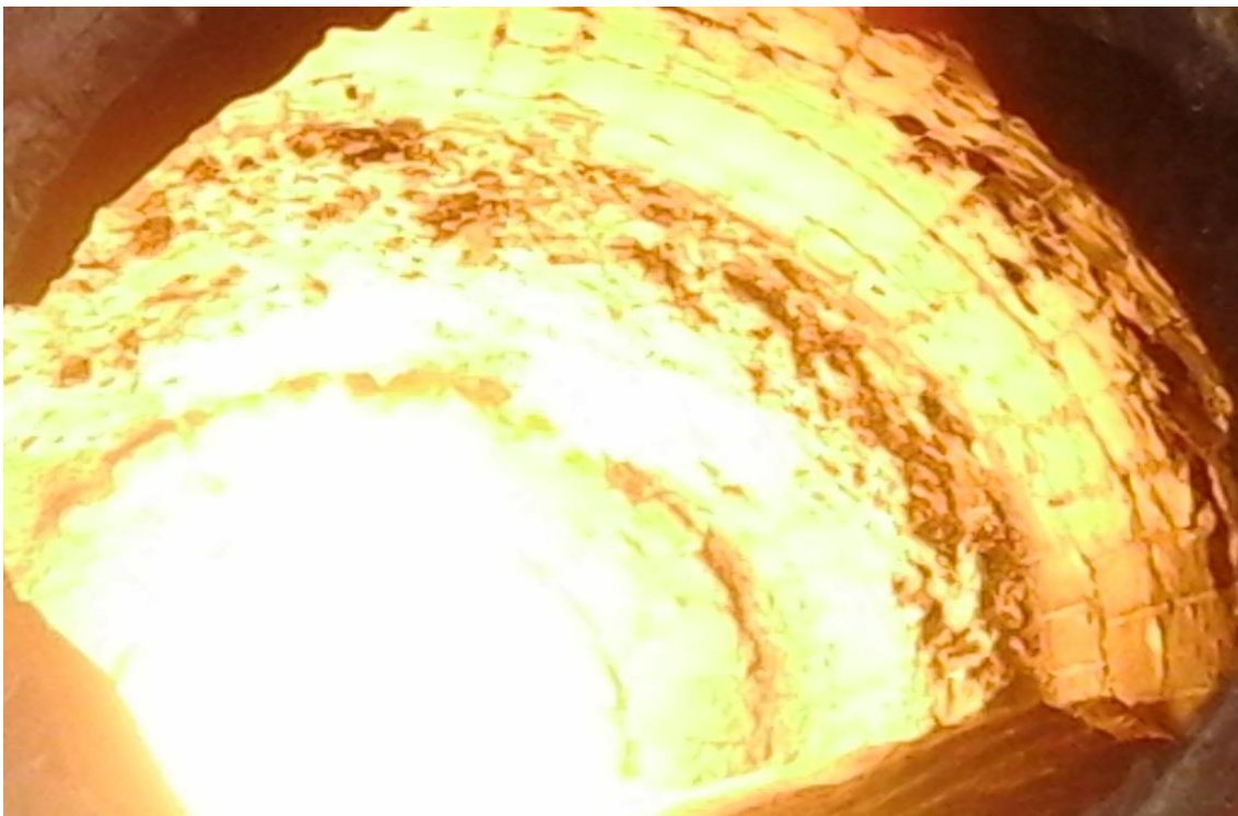
Mineração Tuiuiu - Brazil – Frontier/Four Star Producing gold by pyrometallurgy Inside the smelter furnace we can see the gold volatization – the material stick to the shell are copper gold collector.
