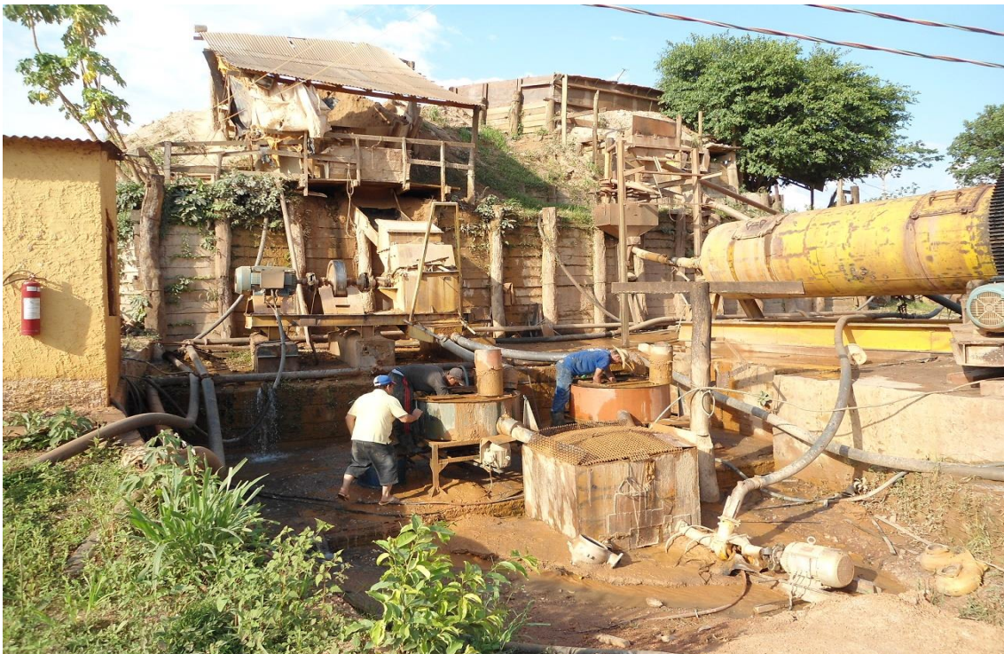
Mineração Tuiuiu - Brazil – Frontier/Four Star Producing gold by pyrometallurgy Existing Gold Mining Operation – Hammer Mill and Centrifuges
