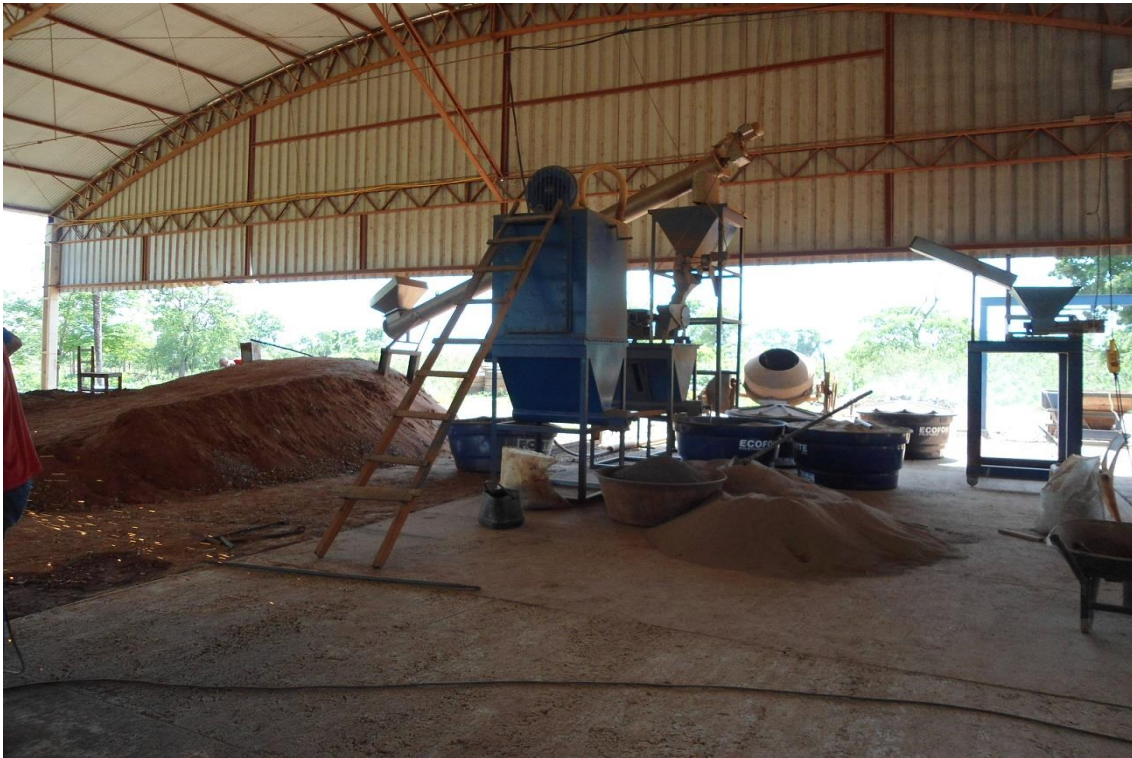
Mineração Tuiuiu - Brazil – Frontier/Four Star Producing gold by pyrometallurgy Concentration Plant
