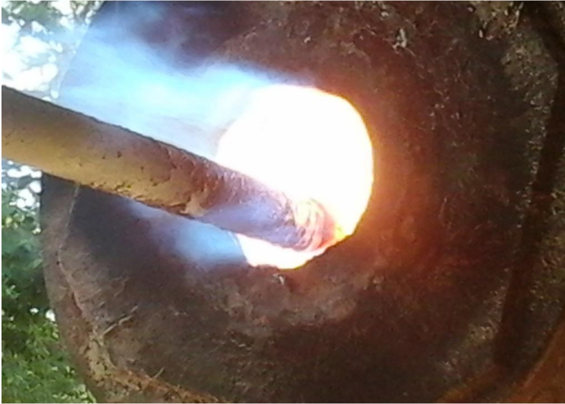
Mineração Tuiuiu - Brazil – Frontier/Four Star Producing gold by pyrometallurgy Volatization of the gold seen in the smoke
