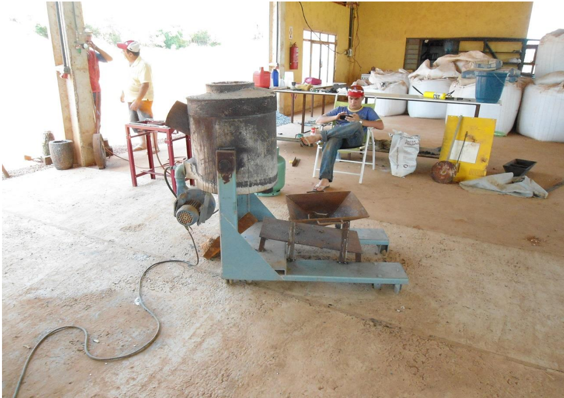
Mineração Tuiuiu - Brazil – Frontier/Four Star Producing gold by pyrometalurgy Refining the gold
